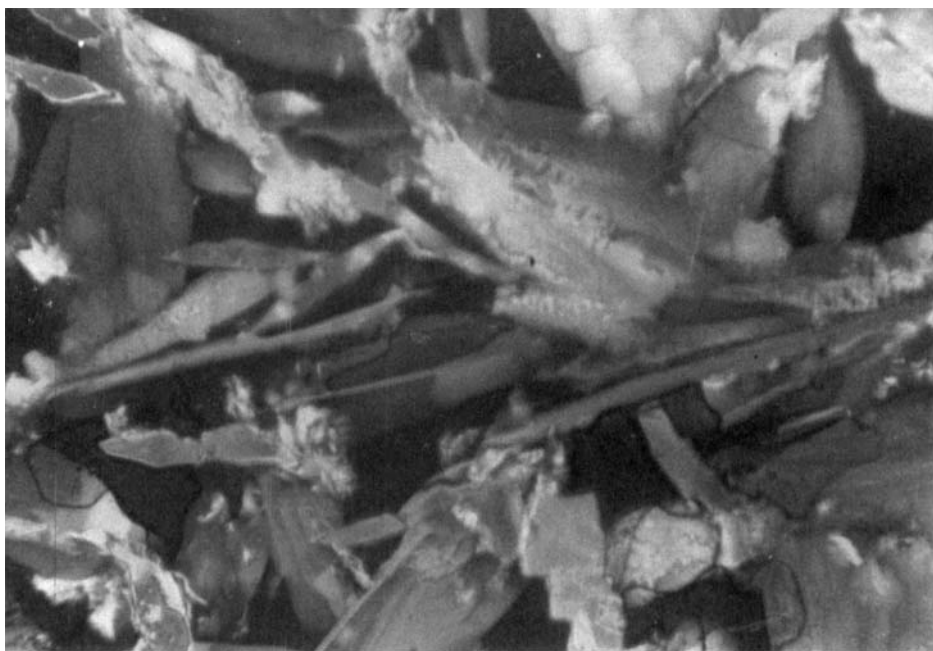
FIGURE 2c Batonnette optical texture (160x) observed at 100°C on cooling the polyester 5. See Color Plate IV.
