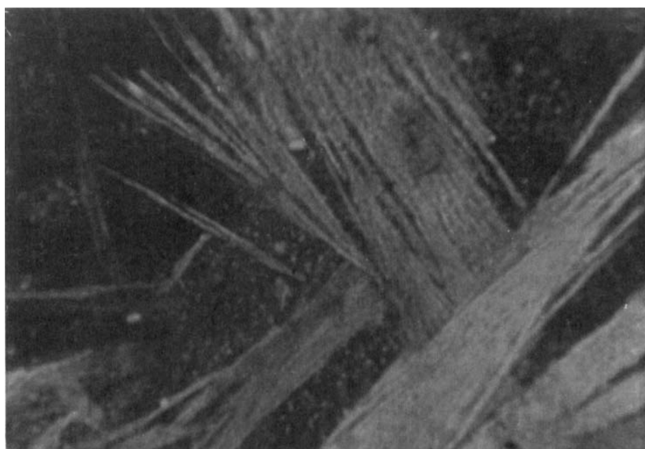
FIGURE 2b Rod-like crystallites (160x) observed at 150°C on cooling the melt of polyester 4. See Color Plate III.
